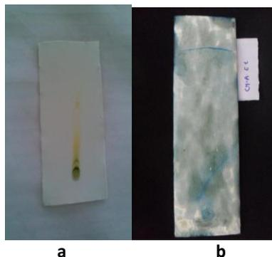
Fig-1: a) Separation of ethanolic algal extract using TLC; b) TLC plate after spraying
